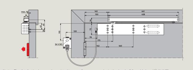
Notice: The distribution box may be omitted in case of a power supply via the door leaf (by cable loop KÜ / LK 12).
