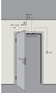
Notice: The distribution box may be omitted in case of a power supply via the door leaf (by cable loop KÜ / LK 12).
