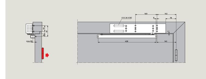
Door closer **TS 99 FL in frame mounted on push side** (transom fixing)
